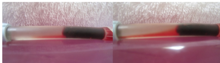
Figure 7 Pre and post control sample (SK enriched group). Image (left) depicts the pre-condition of a typical SK enriched control sample (from sample no. 1). Image (right) depicts the sample following 20 minutes of pulsated fluid only showing only minor changes.
